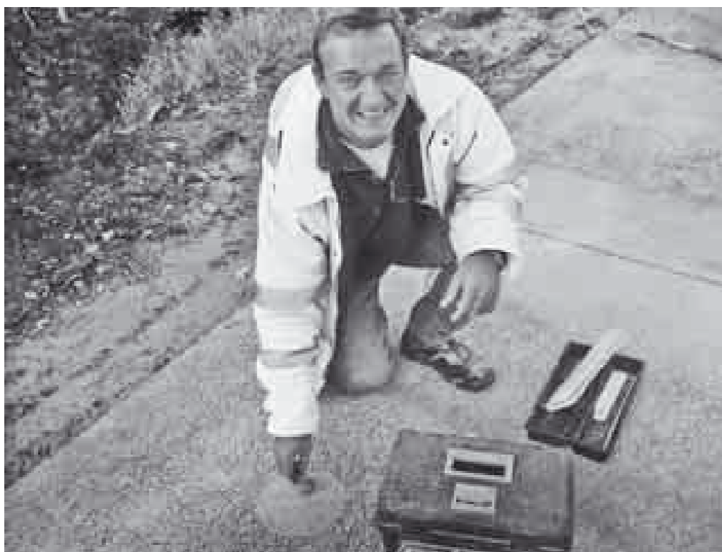
Figure 7: Sand patch test
